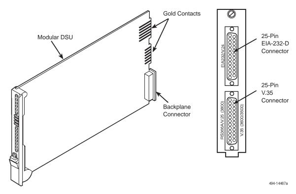
Figure 1. A Modular DSU and Rear Connector Plate
